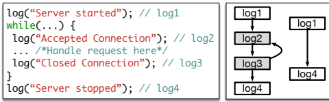
Fig. 6: On the right, LMS control flow paths representation is shown for the code snippet on the left.
